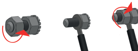
Figure 3. Connecting the unit to an electrical equalizing system
